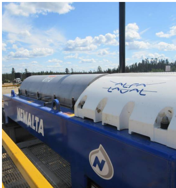
Alfa Laval Lynx 40 centrifuge and stand mobilized to remote client battery site for slop oil processing.
